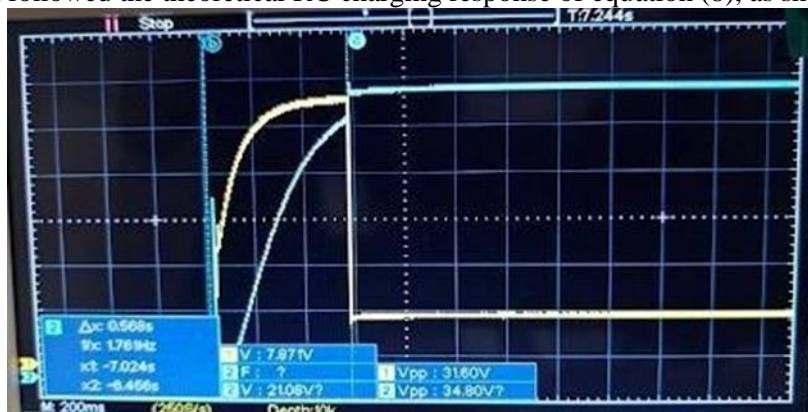
Figure 4: Experimental precharge waveform (200 ms/div) showing exponential DC bus voltage rise toward 84 V pack level.
